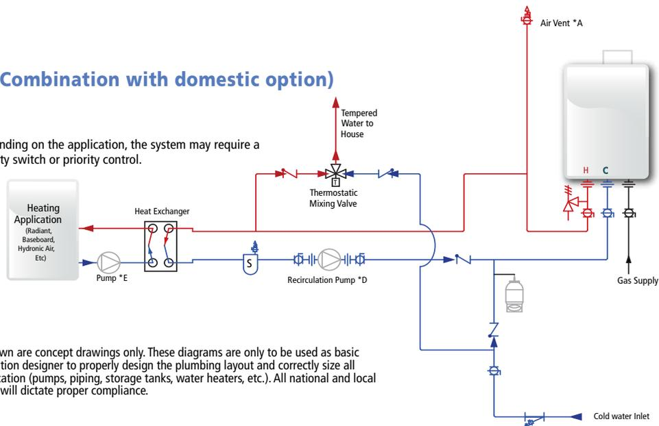
All application diagrams shown are concept drawings only. These diagrams are only to be used as basic guides. It is up to the application designer to properly design the plumbing layout and correctly size all components within an application (pumps, piping, storage tanks, water heaters, etc.). All national and local codes must be followed and will dictate proper compliance.
