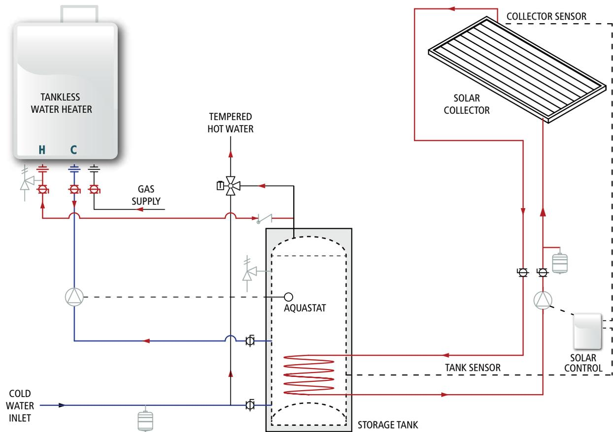
\* The air vent is to be installed at the highest location of the system. The diameter of the pipe leading up the air vent is to be no smaller than the piping throughout the system
