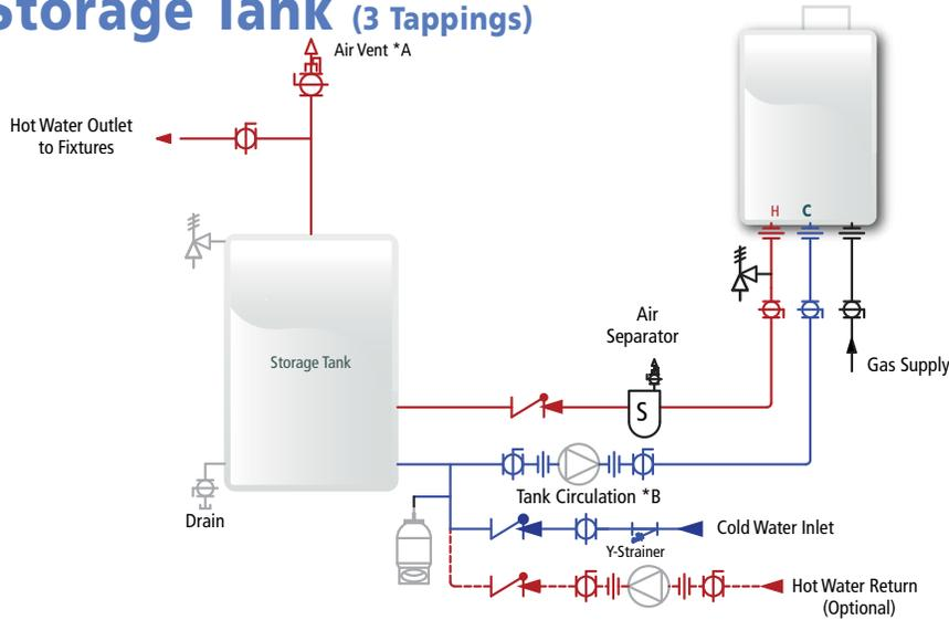
**\*A** The air vent is to be installed at the highest location of the system. The diameter of the pipe leading up the air vent is to be no smaller than the piping throughout the system.
