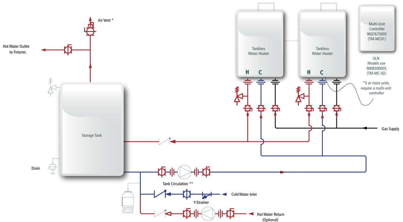
\* The air vent is to be installed at the highest location of the system. The diameter of the pipe leading up the air vent is to be no smaller than the piping throughout the system
