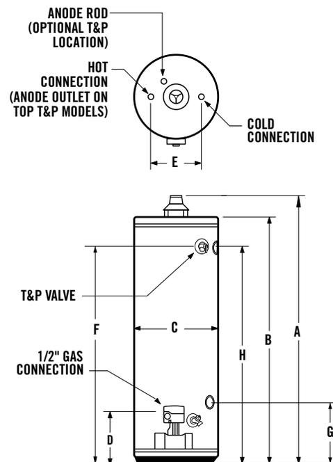
Maximum Hydrostatic Working Pressure: 150 PSI
